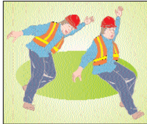
Fig. FH-1A. Most falls in road construction result from slips or trips on the same level.
