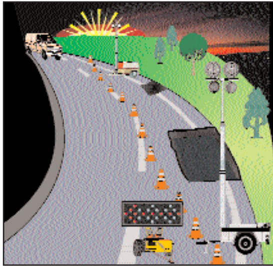
Fig. NW-3. Night work requires many special precautions, including increased visibility and knowledge of surroundings.
