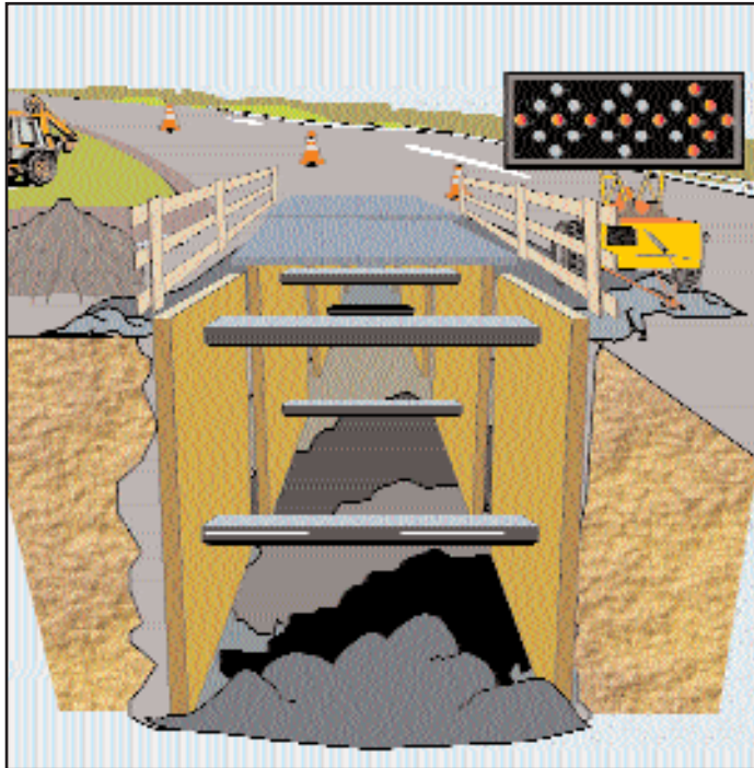
Fig. T-1. An excavation with formwork 15 feet or less from a sidewall is a trench.
