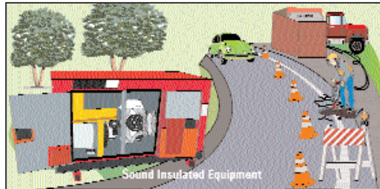
Fig. NH-3. There are many new and effective ways to reduce noise in road construction.
