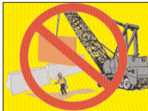
Fig. SC-1B. Keep workers from beneath loads.
