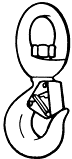
SELF-CLOSING FLAPPER LATCH (SWIVEL HOOK)
