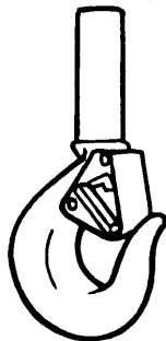
SELF-CLOSING FLAPPER LATCH (SHANK HOOK)
