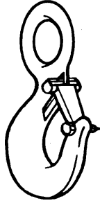
SELF-CLOSING TIPLOCK LATCH (EYE HOOK)
